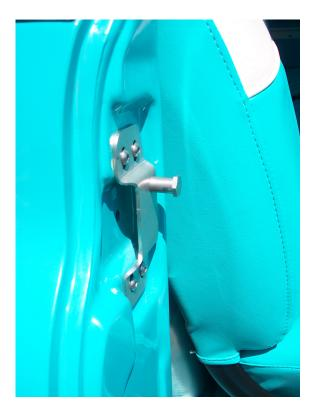
As you close and open the door, feel for "climbing" or "dropping" and then adjust accordingly. The striker also has in and out adjustment.
