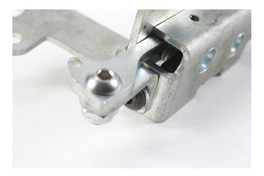
The 90 Degree lock lever bracket mounts to the bottom of the latch using the 1/4-28X3/8 Black Button Head Bolt and Lock Washer. Attach the lock lever to the bracket using the 1/4-20 Stainless Button Head Bolt and Locking Nut. The lock lever should be able to rotate smoothly.
