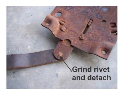
Note: This is a good time to liberally lubricate all moving latch and lock parts before its final placement in your door. We recommend dry-film lubricant or lubricant with graphite. Otherwise, marine grease or white lithium will work as well.
