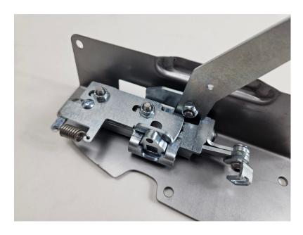
7. Locate the rivet holding your inside door handle strap to your factory door latch. Grind this rivet and separate the strap from the latch.
