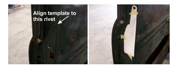
Trace around the template. Do not trace around the hole alignment piece. Do not trace along the edge lined up with the corner of your door. Instead make a mark at the top and bottom of the template where they meet the corner. From those points measure 1 ¾" toward the center of the door. Mark these points with a pen or marker. Using a straight edge connect your points and you will have your cut line. Make your cutout
