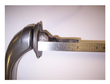
Alternatively, you can securely install the latch in your door. Then measure the distance from the outer skin of the door through the exterior handle hole and into the handle receiver on the latch. You do not want the shaft to be long enough to pass through the shaft receiver and hit the latch body itself. This will cause rough operation.
