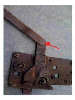
11. Attach the interior door handle strap to your new latch assembly using the 10-32 screw and locking nut provided with your kit. Do not over tighten as this is a pivot point and must remain free to move. Next, slide everything into the door through the hole you cut for the latch assembly. Reattach your interior door regulator in its stock location. Reattach the latch and plate assembly to the door.
