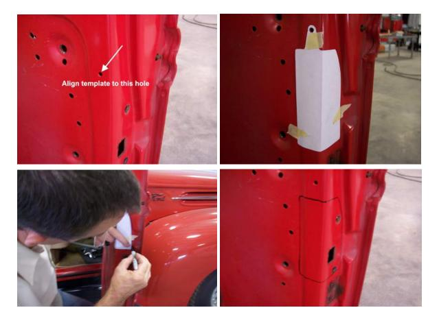
6. With the latch removed from the latch plate, place the latch plate against your door. Align the latch plate so the top of the latch plate is approximately 3/32" from the bottom of the alignment hole. Mark the holes for attaching the plate to your door. Remove the latch plate and drill the holes using a 1/4" drill bit.
