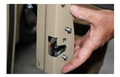
8. Attach the plate securely to the door making sure to use the 1/4-20X1/2 Stainless Button Head Bolt in the upper mounting hole on the jam plate. Tighten the 2 bolts holding the latch to the plate. Reinstall your exterior door handle. Insert the provided 1/4-20X1/2 stainless button head bolt in the center mounting hole. If your handle does not align with the handle receiver on the latch, remove the latch and plate assembly and adjust the position of the handle receiver accordingly.
