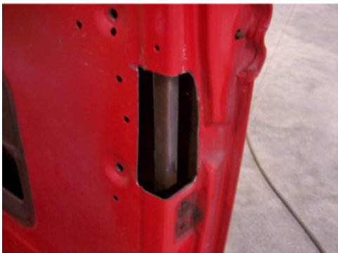
Fig. 5a Carefully cut hole for latch assembly
