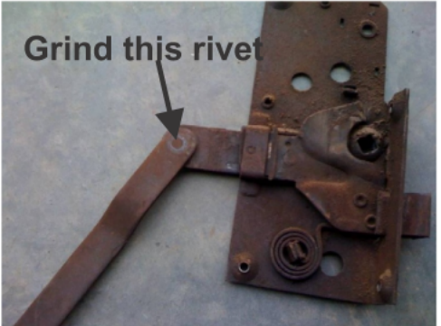
Fig. 7 Grind rivet and separate strap from latch.
