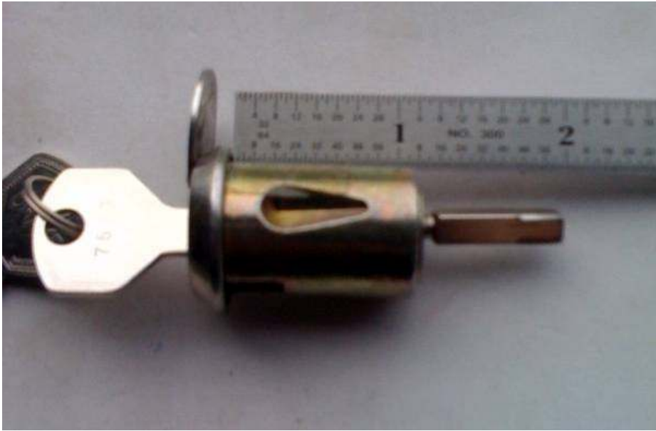
Fig. 9 Measure from the bottom of the lock cylinder bezel 1 \frac{3}{4} " and cut lock cylinder shaft. If you are installing lock cylinders in the drivers side it will need to be cut at 1 \frac{7}{8} ". It is necessary to purchase our installation kit for installing lock cylinders in your drivers side door.
