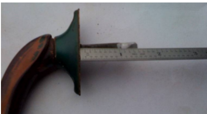
Fig. 1 Measure 1 17/32" from base with no gasket. Mark and cut shaft. If you are using a gasket you will need to add the gasket thickness to the length of the shaft.
