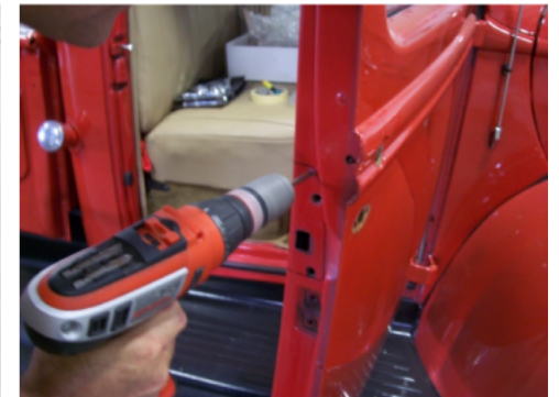
Fig. 5 Drill 1/4" holes in each corner
