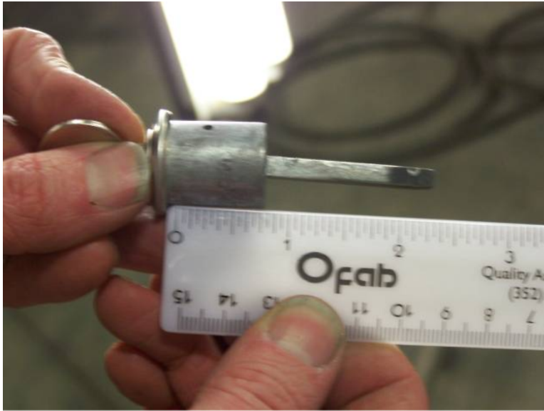
Fig. 7 Measure (Coupe) 2 1/2" or (Tudor) 2 1/16" from base with no gasket. Mark and cut shaft. If you are using a gasket you will need to add the gasket thickness to the length of the shaft.
