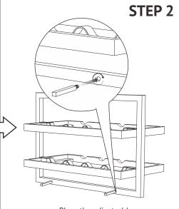
Place the adjuster(s) note: Winerack A and C have 2 adjusters
