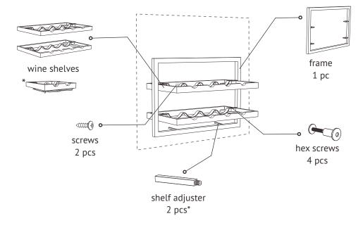
\*note : - SHELFMATE Winerack A and C have 2 adjusters. B, D and E have only 1 - Only SHELFMATE Winerack D has a glass holder
