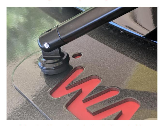
Step 3) Place the rubber washer on the threads of one side of the support rod. This will be the side that goes into the wing extension. Install this end of the rod through the bracket and extension, and loosely tighten it up
