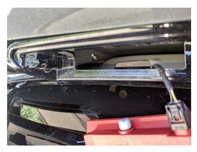
Step 8) Push your support rod end into your spoiler and tighten it down, snugly. Be sure to use a nylock nut or locking washer to keep it secure.
