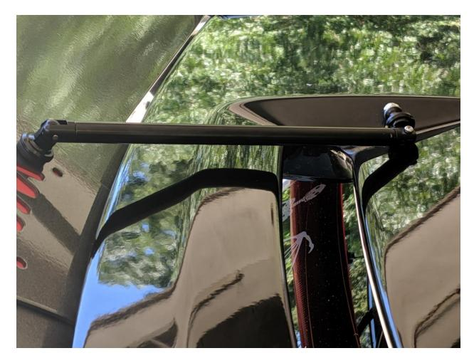
Step 4) Roll the support rod to the location that you want to attach it to the spoiler. I chose to mount it on the inside of this part, but it can be mounted in any location that is accessible from behind the third brake light.
