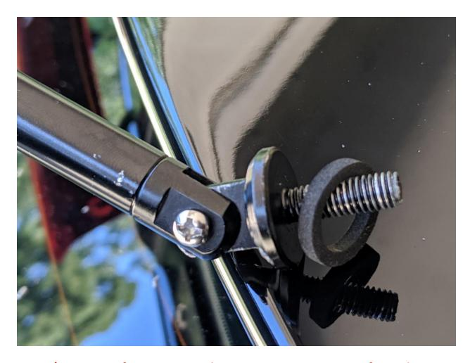
Step 6) Use your foam EVA washer to protect your paint from the support rod hardware. This is used on the side that bolt to your spoiler
