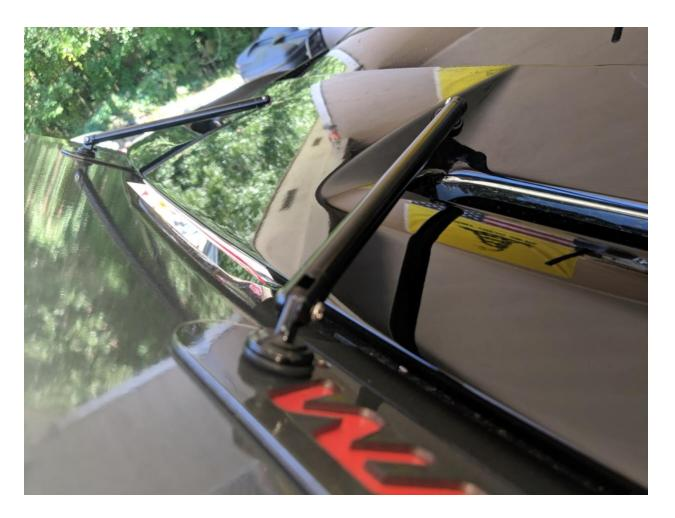
Step 9) Tighten up your support rod end that attaches to the extension. The rubber bushing should be smashed about halfway and will help absorb some of the shock between the extension and the wing. You can now replace your third brake light and the installation is completed.
