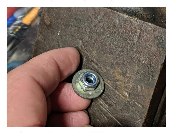
Step 7) Use super glue, or some kind of adhesive to mount your washer to the back of your nut. This will help you to maneuver it in place. Your washer should be the same size or bigger than the surface area that you're mounting to on the outside of the spoiler.
