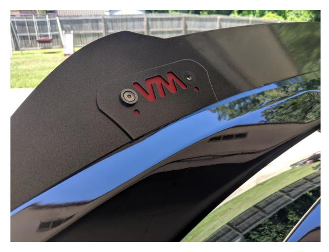
Step 1) Remove the inner bracket bolts on your wing extension
