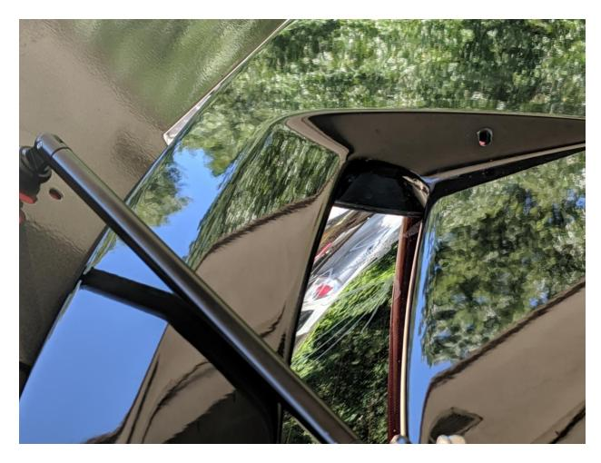
Step 5) Drill your hole. I used the 1/8" bit for a pilot hole, to make sure I was lined up correctly. Follow that hole with the 1/4" bit. I drilled a slot in mine to have a little adjustability up and down with the support rod hardware.
