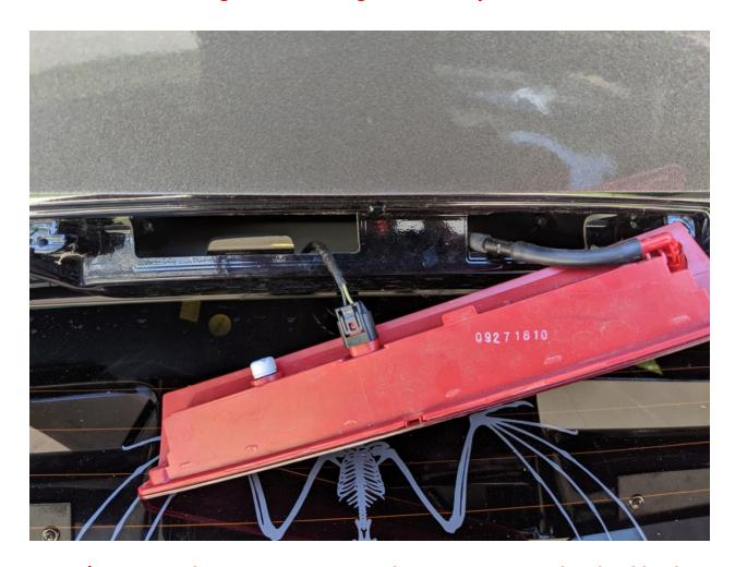
Step 2) Remove the two Torx screws that are securing the third brake light, and remove the third brake light. You can just leave it hang in place.
