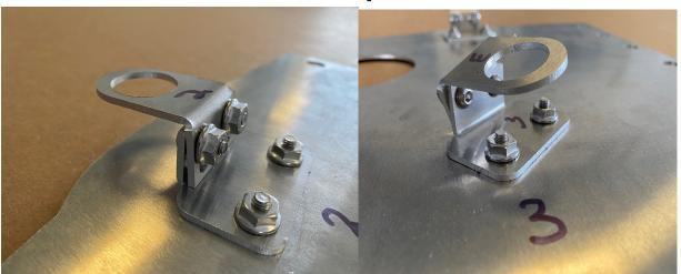
The brackets are labeled (1,2,3). Match the brackets using the pictures above as a reference. They have to be installed properly or the cover will not mount correctly. Turn this guide over for a cropped view.
