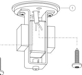
Shorten the cable to the required length for hanging the pendant light and remove wire insulation according to the diagram. The cable (+) and metal braid (-) will serve as conductors for electrical wiring.
