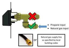
2. Lay the burner upside down on a flat, soft surface to avoid scratching the polished metal. Ensure the correct orifice is installed for the fuel type you are using (see Crystal Fire user manual included with burner for orifice sizing information) Attach the included metal flex hose to the burner.
