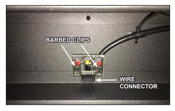
Figure 15 Remote Receiver Replacement
