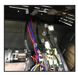
Figure 11 Seven Electrical Connections required for Heater/
