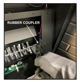
Figure 12 Rotisserie Rod Removal
