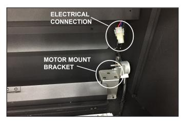
Figure 14 Motor Replacement
