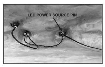
Figure 4 Light LED Connection on Bottom of Log Ember Bed
