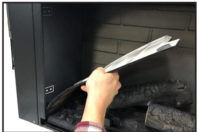
Figure 4.12 Decorative Side Panel Removal
