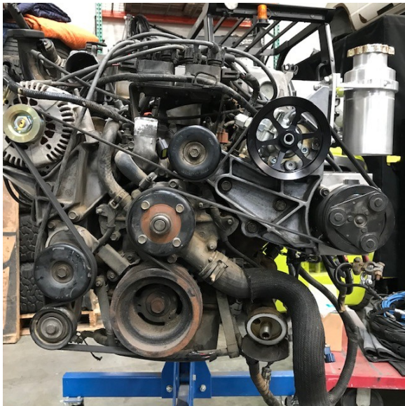
Belt routing with AC (Belt # 6PK2375)
