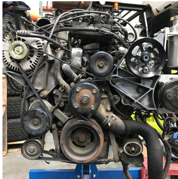
Belt routing without AC (Belt # 6PK2082)
