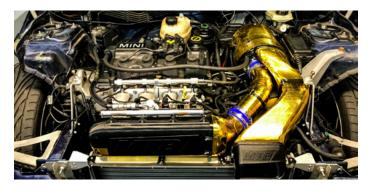
To increase the compression (12:1), the cylinder head and engine block have been modified as well. In addition, I have fitted an improved camshaft.
