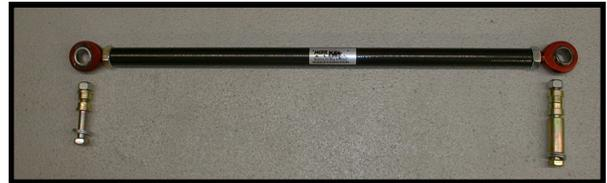
Please note. There has been some confusion about where this trac bar mounts. It is for the front axle only on Jeep® YJ Wrangler vehicles. Do not even think about installing this on a XJ Cherokee, TJ Wrangler or on the rear of a YJ.
