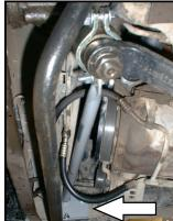
This steering brace fits 1987-2001 Jeep® XJ Cherokee vehicles with power steering, and 4.0L engines. It is designed to bolt into existing holes in the chassis, with minor drilling, and clamps to the steering box housing just above the sector shaft/pitman arm.
