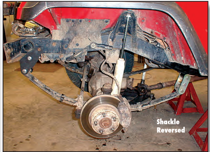
This photo is the same YJ with our S.R.S.™ installed with optional Lubeable Shackles (# LS9040). Notice how the axle is forward from the stock location.
