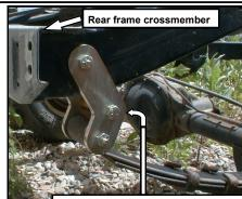
This is the proper location for the bolt-in center brace. The long leg up, center brace forward. This way, the shackle can clear the rear crossmember on suspension compression.
