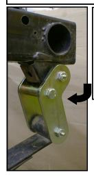
This is the proper way to install the shackles on the FRONT of the YJ. The long leg down, bolt-in center brace back. This way, it acts as a "Anti-Kick-Back" shackle.
