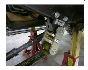
This is the proper configuration for the shackles. On some applications the bolt in center brace may need to be left out. This picture shows the shackle in a S.R.S. set up.
