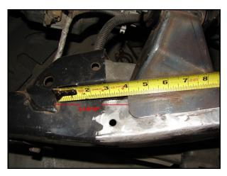
Passenger side: Measure from the Upper Control arm bracket to the back side of the JM700 Mount. This measurement should be **3-15/16**"
