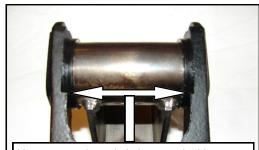
You may need to grind clearance in this area to allow the BombProof  $^{\text{TM}}$  mount to fit into the factory "fork". More common on YJ's.
