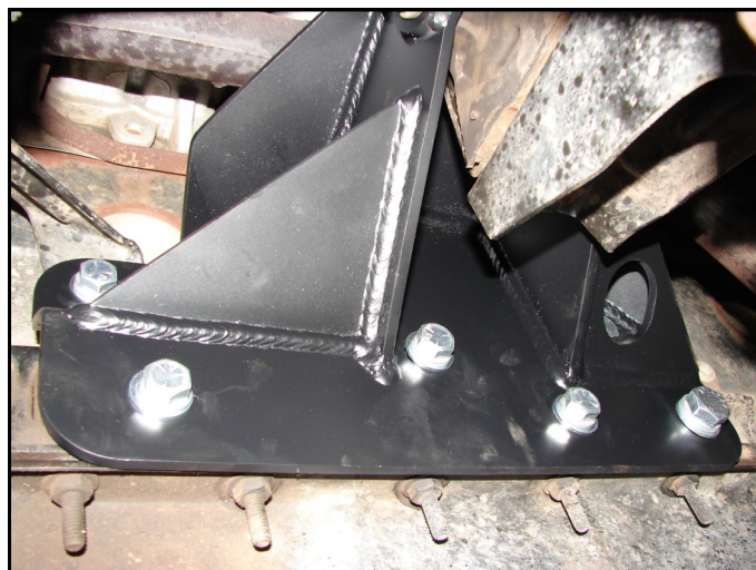
DS Block Bracket Installed
