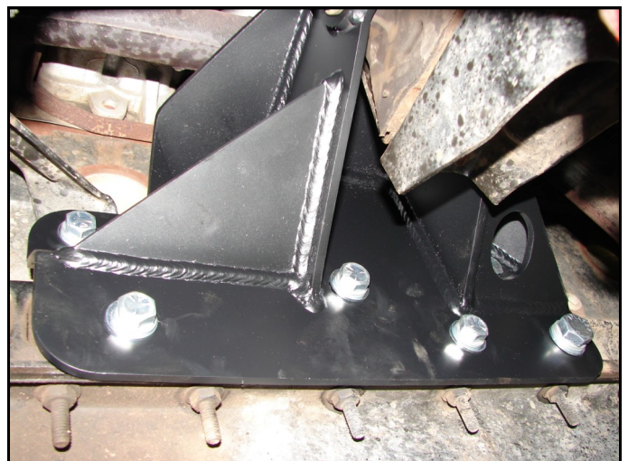
DS Block Bracket Installed
