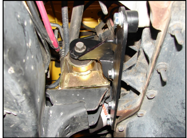
PS Block Bracket Installed
