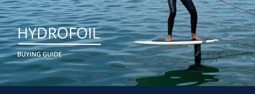
A hydrofoil is a board with a wing attached to it by a mast. You stand on the board with the wing submerged in the water and when you start moving, getting water traveling fast enough across the wing, it generates enough lift to float the board free of the water so you start flying!
