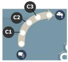
In Automatic mode, pressing and holding down the allows changing the adapted thermoregulation curve.
