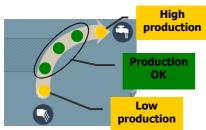
The production level is given by green and yellow indicator lights. If no green indicator light is lit despite a production set to the maximum, then it is necessary to check the salt ratio.
