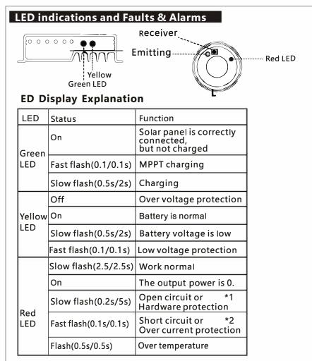
\*1.If the controller is in transport mode, the red LED is super slow flash(0.2s on/5s off),the green and yellow led is off. \*2.Detailed fault information can be read by S-Unit remote controller.
