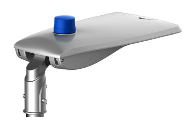
The SL2 Series LED streetlight range offers a reliable and modern LED solution for new installations and retrofits. The high output Nichia LED chips can utilise a 'Batwing' distribution lens system to ensure a wide and even spread of light, which is perfect for carparks and roadways. The smooth top surface limits the build up for dirt and debris. With the addition of Casambi wireless control, users are easily able to interact and customise their lighting environment.
