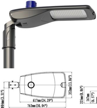
The SL2 Series LED streetlight range offers a reliable and modern LED solution for new installations and retrofits. The high output Nichia LED chips can utilise a 'Batwing' distribution lens system to ensure a wide and even spread of light, which is perfect for carparks and roadways. The smooth top surface limits the build up for dirt and debris. With the addition of Casambi wireless control, users are easily able to interact and customise their lighting environment.
