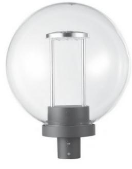
The PT6 Series is a stylish edition to Integrated Powers' family of heritage and contemporary designed poletop fittings. With its classic look and indirect lighting, the PT6 provides visual comfort and easy viewing. The PT6 allows for the base and gear compartment to be removed for easy access to the driver.
