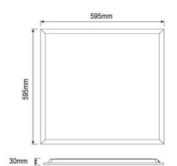
The PBC Series LED Panels balance high output with clean, even light distribution. These panels not only reduce glare, but include flicker free drivers adding an extra layer of visual comfort in the workplace. They are a stylish troffer replacement for standard grid ceilings. Perfect for either retrofits or new buildings. Through the power of Casambi smart technology, users are able to customise their desired outcome though luminaire dimming, grouping, scheduling and so much more.
