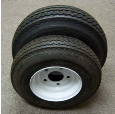
Front Tire = 4.80 x 8, C-Rated, 6-Ply **Rear Tire = 5.70 x 8, D-Rated, 8-Ply
