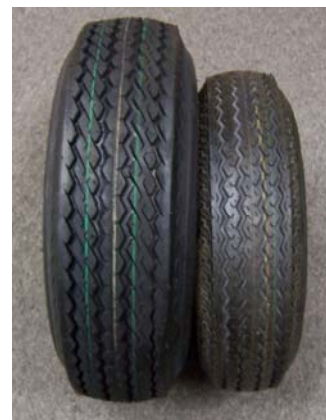
Right Tire = 4.80 x 8, C-Rated, 6-Ply **Left Tire = 5.70 x 8, D-Rated, 8-Ply
