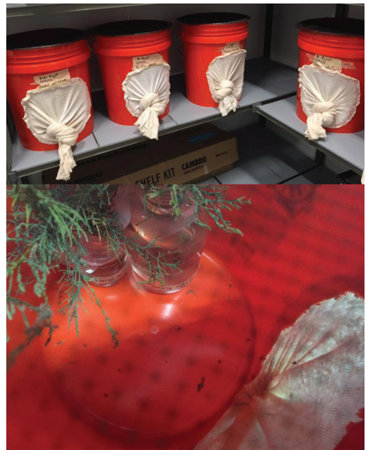
Figure 1. Bucket cage design. Top: A 5-gallon bucket with 30 x 30 cm front panel removed. The front face was enclosed by securing a 60 cm length of cylindrical stockinet. Bottom: Salt cedar cuttings nested in water for conducting a bioassay.
