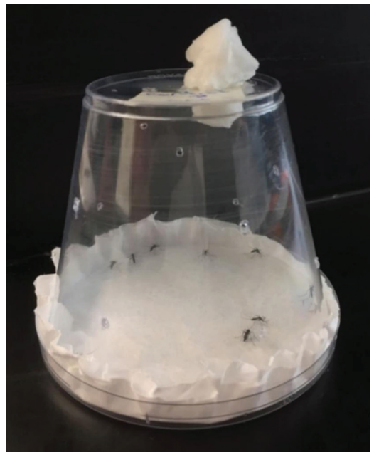
Figure 1. Bioassay chamber constructed of a Petri dish base, a pesticide-treated filter paper nested in the dish, and a ventilated polystyrene cup with sucrose solution wick, and containing 15 non-blood-fed, 5-7 d old female Aedes albopictus (Skuse).
