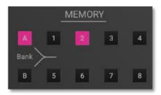
The Memory section offers 16 patches for fast preset accessing. Two banks of 8 sounds each are available.
