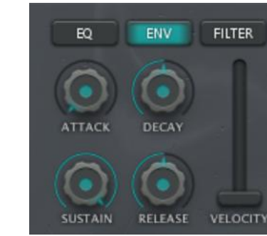
Envelope Panel Standard Attack, Decay, Sustain and Release controls along with a velocity sensitivity slider
