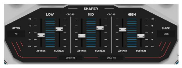
Attack - Controls the level of the transient signal in each band.
