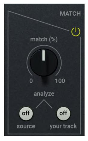
**Match Power** – Turns on/off the Match section, which enables you to match the frequency of your track to the source track.
