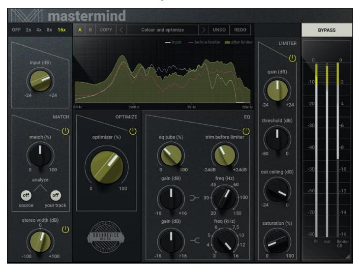
Input - Controls the gain of the input from -24 to +24 dB
