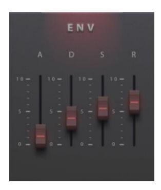
Envelope that generates the control voltage applied to the VCF and VCA. Envelope has 4 parameters:
