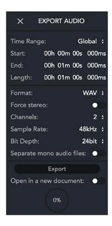
With the "Separate mono audio files" option activated, each channel is exported to a separate mono audio file (the channel number is appended to the name of each audio file).
