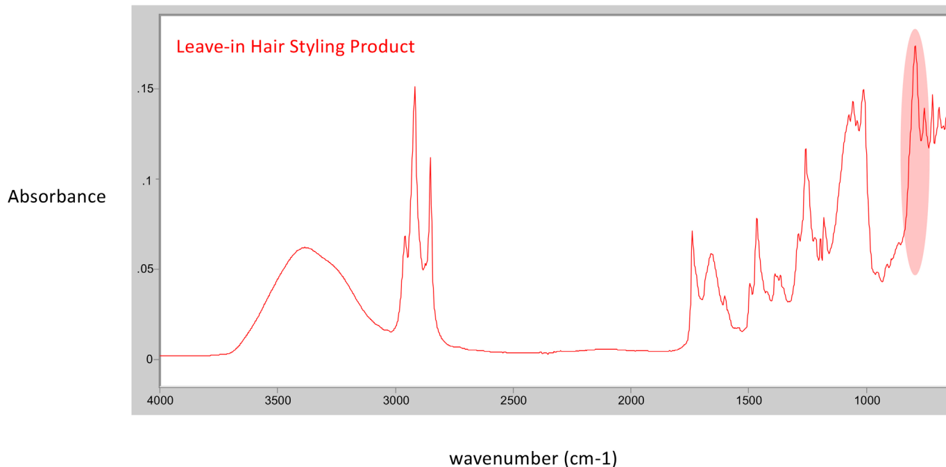
FIGURE 3. FTIR spectrum recorded on leave-in hair styling product used for this study. The red ellipse shows the IR marker that was used to follow specifically the leave-in styling product used to treat the hairs. Indeed, there is almost no skin contribution in this spectral area. The band around 800\text{cm}^{-1} was used in this study to investigate over time the deposition of leave-in product at the surface of different skin locations.
