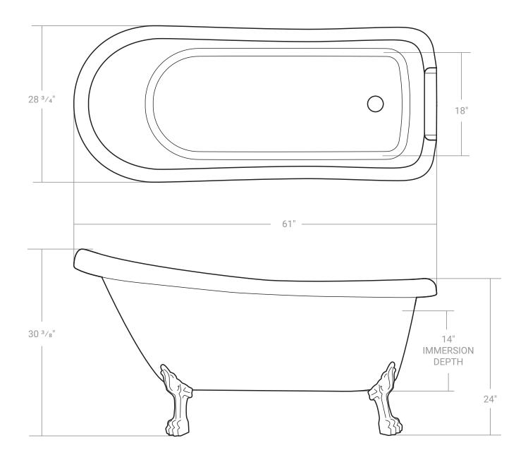
\*All measurements are + 1/4" \*Drawings are not to scale
