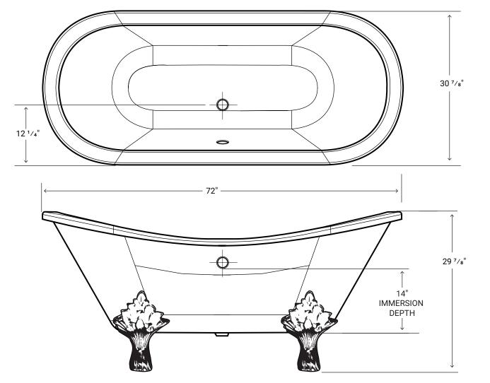
\*All measurements are + 1/4" \*Drawings are not to scale
