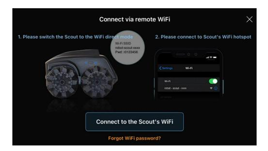
After it powers up, the Wi-Fi shall stay in the "Wi-Fi Direct" Mode, which is the out-of-factory condition. Scan Wi-Fi around you. There should be Wi-Fi with the SSID name **robot\_scout\_XXXXXX**. This is Scout.
