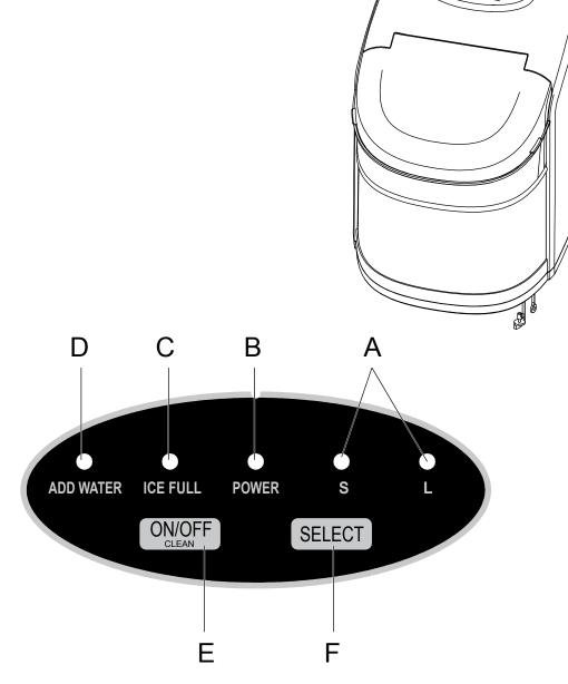
Start the self-cleaning program: Plug on the unit, then press "ON/OFF" button for more than 5 seconds to enter the self-Cleaning program. Self-cleaning program need 30 mins. When the program is over, please drain out the water and clean inside.
