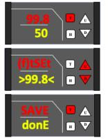
When main screen is active, Hold T button for 2 seconds
