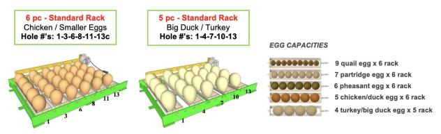
Racks must be adjusted for larger eggs. If the egg is too large, it may fall down during turning.
