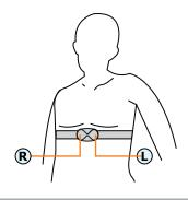
Wear the strap slightly below your chest. Place the Sensor in the middle of your body, where the electrodes are placed against your skin must be pressed.
