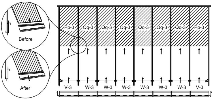
Insert the second row of panels into the lower groove on the rafter. Slide panels until they reach the aluminum pieces between the panels and gently tap on the panel to guide it into the aluminum groove. Use a spatula if needed to make it fit. Insert two (2) Pp-3 on either end, then insert the Qq-3 panels.
