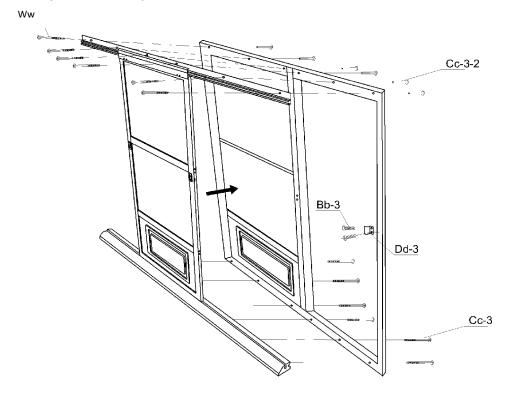
Anchor the solarium to the deck or floor securely using screws and shields supplied. See diagram below.
