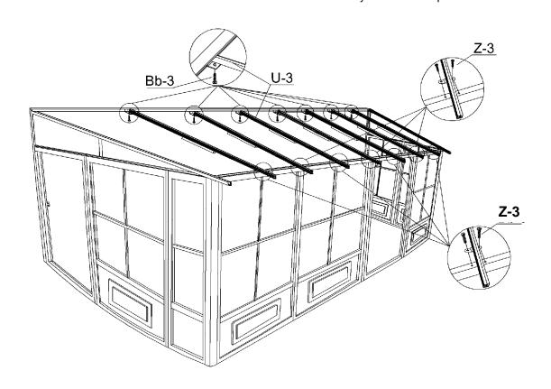
Remove protective film from two (2) sides of each panel and make sure the top side of the panel faces the sunlight. Insert and slide on the top groove of the rafters all the way to the end. Pp-3 should go first and last with the Qq-3 panels in between.
