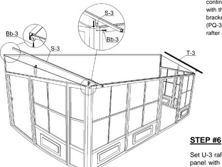
Set U-3 rafters over the middle of each panel with Bb-3 screws at the top and two (2) Z-3 screws over the brackets on frame manually. Set U-3 rafter on each joint and use Z-3 screws manually. Do not use power drill.
