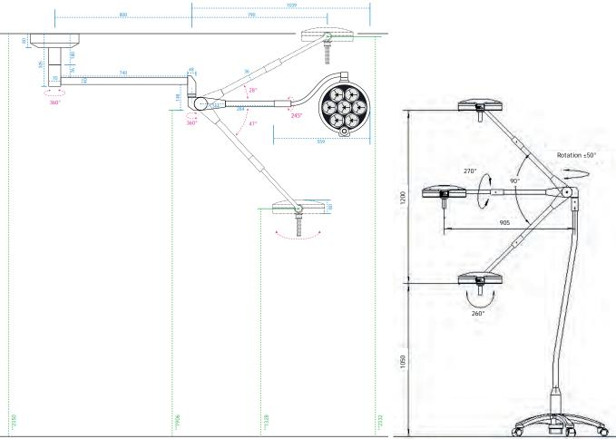
\*\*Dimension suggestion. For specific applications or environments, then mounting bracket should be installed at a height so that, when fitted, the lighthead is as near to the required position as possible
