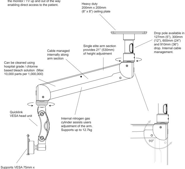
Supports VESA 75mm x 75mm and 100mm x 100mm compliant LCD/TVs
