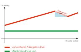
The resulting insufficient regeneration of the dryer leads to a gradual increase in the moisture content of the compressed air. Compressors with simple adsorption dryers are thus not suited to run such machines. The innovative membrane-drying unit from Dürr Dental means that there is no need for regeneration times. A constant supply of dry, compressed air in continuous operation is guaranteed.
